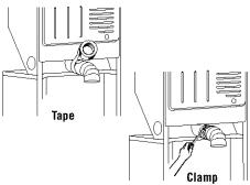
**STEP 4.** Connect vent to elbow. Tape the joint with duct tape. Tighten clamp.
